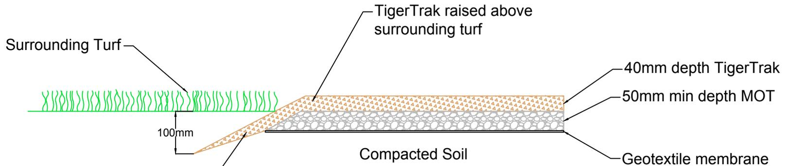
'Chase' or groove at perimeter to allow Tiger Trak to chamfer down and then be covered in topsoil. (No terram or stone in the chase, to allow grass to grow through the TigerTrak here.)
